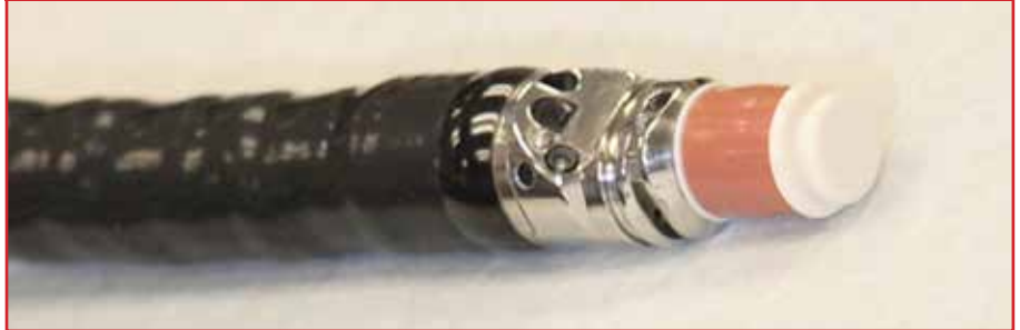
Figure 1. Electronic radial echoendoscope (GF-UE260, Olympus Co., Ltd., Tokyo, Japan) can provide 360-degree cross-sectional images and Doppler study
